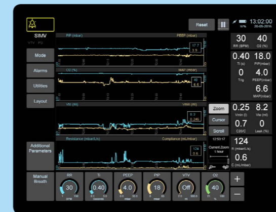
All parameters are trended and can be shown on the trend screen. A maximum of 14 days can be recalled and then scrolled and zoomed.
