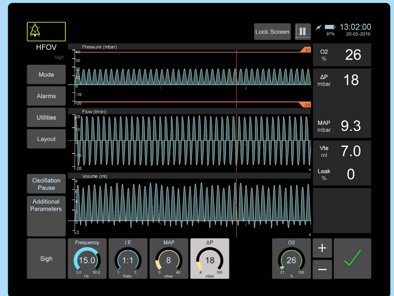
Switching to HFOV is a button-push away, and does not require any changes to the patient circuit. Parameter controls have changed to reflect the new mode. The 'Additional Parameters' button can display secondary controls for this mode. Selecting any parameter activates the + and - keys to adjust the parameter value.
