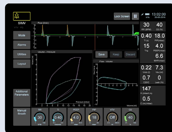
A lung mechanics screen shows additional data - in this case two loops. A secondary column of data can be shown when required.
