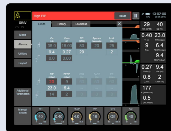
An alarm screen gathers all alarm settings in one place. Alarming parameters will show as cyan, yellow or red depending upon priority.
