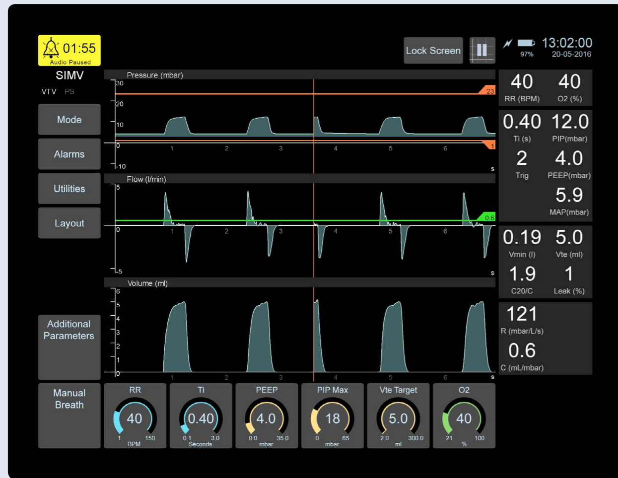
This ventilator has been set up to show SIMV with three waveforms. In this example, the audio alarm has been pre-silenced and a countdown timer within the button shows the remaining time. By default only the necessary parameters to control SIMV are visible.
