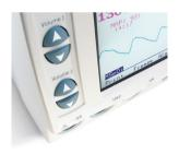
When monitoring twins, independent volume controls facilitate transducer placement by allowing both heart rates to be heard at the same time.
